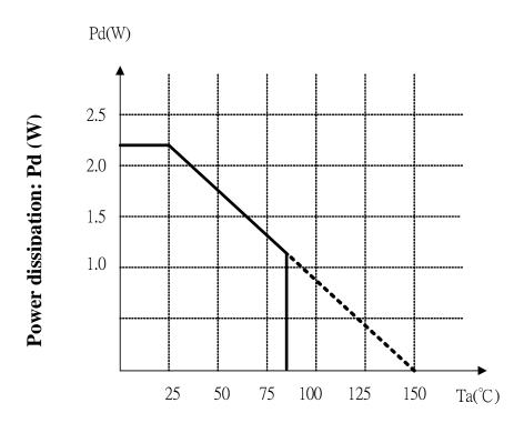
Ambient temperature : Ta ( $^{\circ}$ C)
